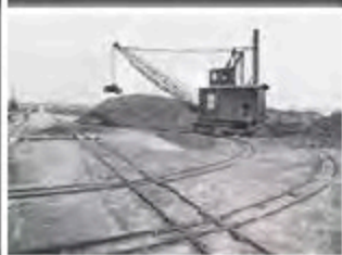
1894 - THE FIRST CRANE: A STEAM-POWERED CLAMSHELL CRANE FOR COAL.
