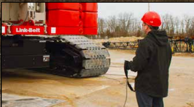
Complete counterweight removal/assembly from ground level
