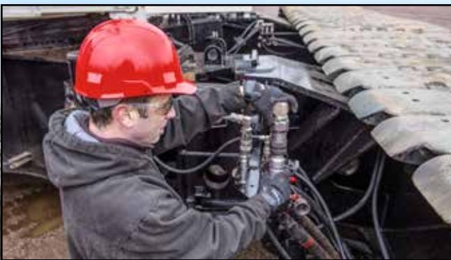
Hydraulic quick disconnects for effortless hook-up
