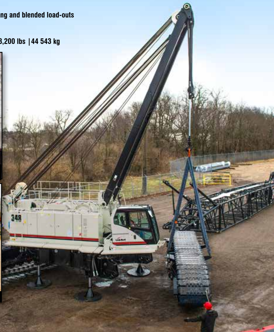
Complete counterweight removal/assembly from ground level
